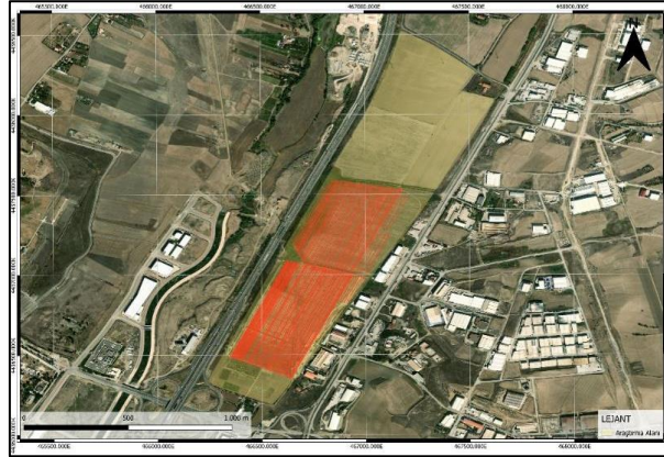
Figure 5. Drawing flight blocks with QGIS program.
