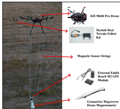
Figure 4. Components of the UAV magnetic system.
