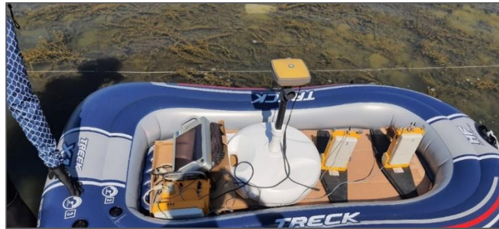
Figure3 GPR measurement setup with 200MHz antenna
